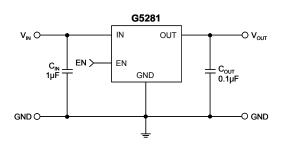
Note: Recommend connecting the Thermal Pad to the GND for excellent power dissipation.
