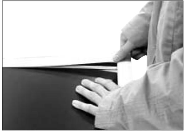
4. Cover the panel with your hand so that it is not scratched. Then, pull up the cabinet corner side.
