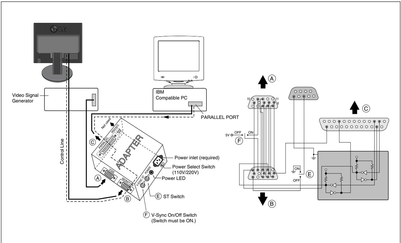
**Figure 1. Cable Connection**
