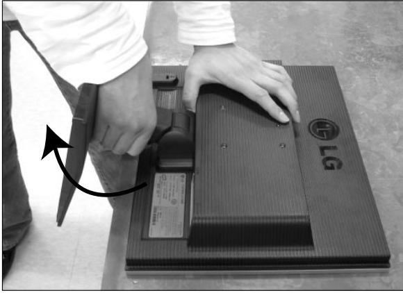
In assembly state, rotate stand body to upper side.
