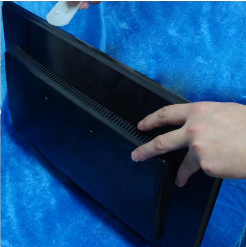
**Note: The positions of the clips on the rear cover are as follow. There are some small gaps between CLIPS.
