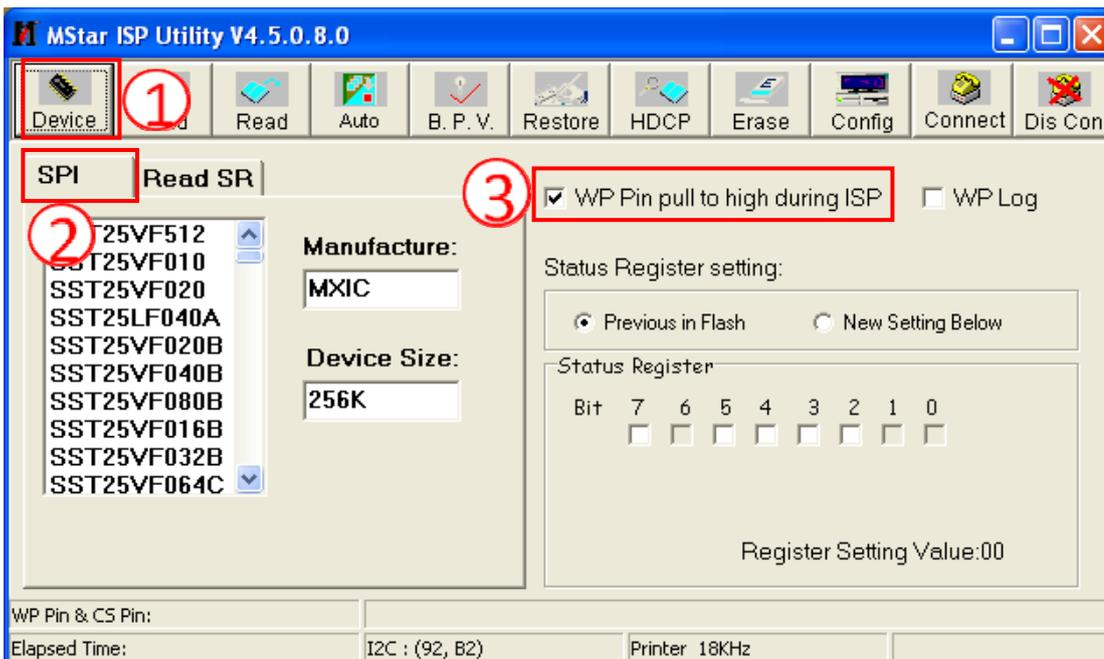
4.4. Connect to the monitor. Click “Connect”. If the tool communicate with monitor successfully, the tool will detect the flash type of monitor.
