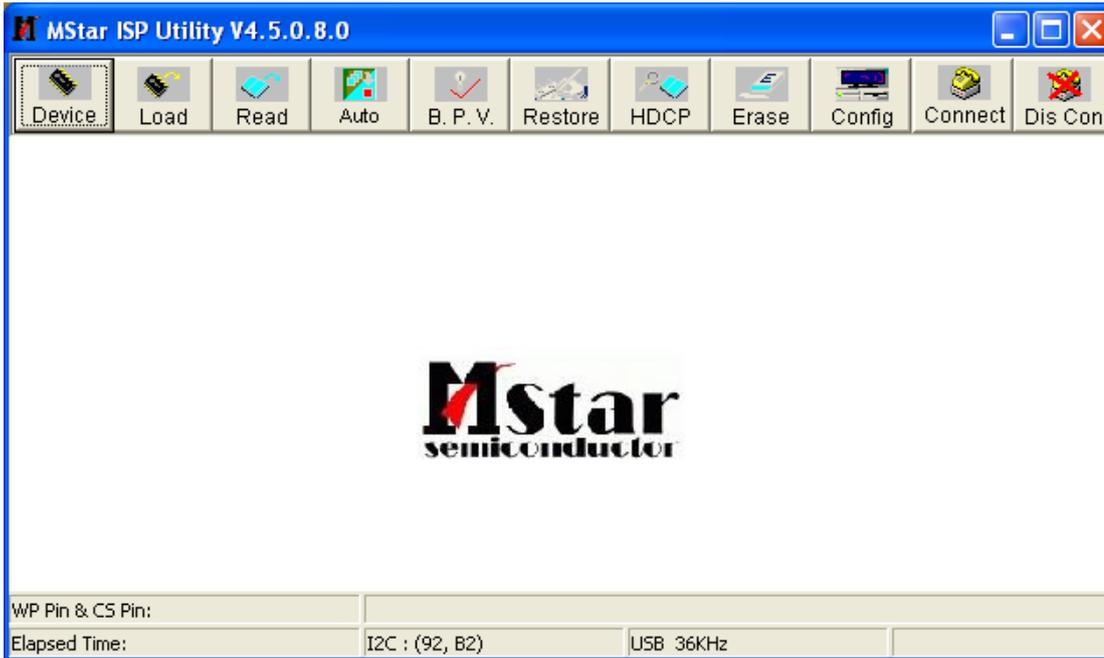
4.3. Set the parameters in "Device" window. Tick "WP Pin pull to high during ISP".
