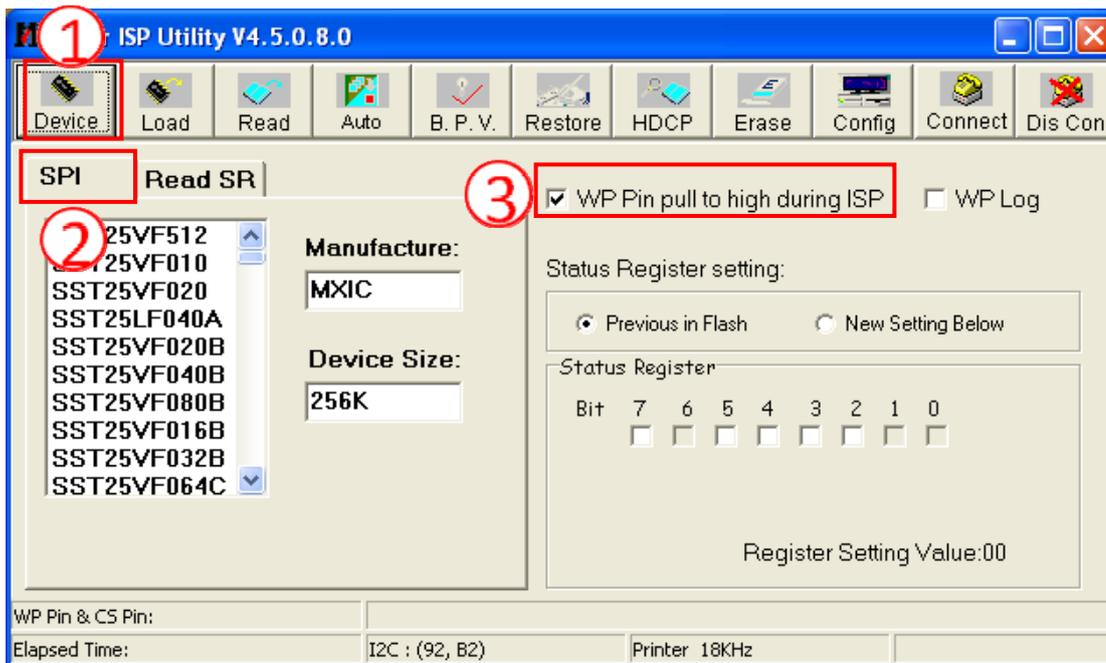
4.5. Connect to the monitor. Click “Connect”. If the tool communicate with monitor successfully, the tool will detect the flash type of monitor.
