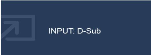
Press the **ENTER** key to toggle between different PC video signal inputs that may be connected to your monitor. The setting will take effect immediately. The setting will take effect immediately. The setting will take effect immediately.
